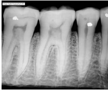
Figure 1: Standard teeth phantom image, 150ms exposure with 60keV X-ray energy
