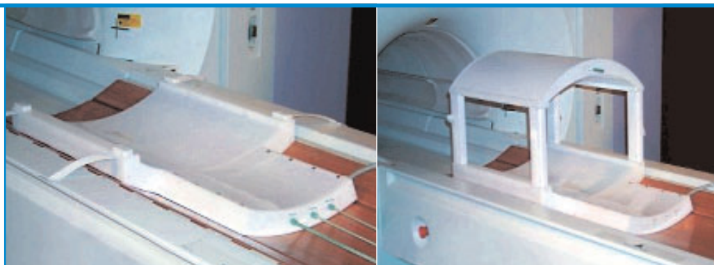
Figure 2: The opened and closed 3\text{H}/1\text{H} MR coil with green tuning and matching rods at maximum size for a 1.5 Tesla Siemens scanner. The design allows the investigation of large-size humans within the limit of the 60-cm opening of the MRI scanner. The coil inside the housing is a variation of a volume-type coil, where the electronic connection between the upper and lower parts of the wires of the coil is performed within the distance-adjustable spacers.
