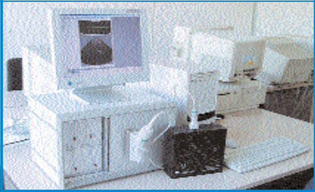
Figure 2: Digital phased-array system connected to a probe and a PC with display.
